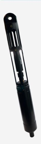
The aquaMeasure BGA is a compact, wireless underwater sensor that measures BG Algae, temperature and tilt in realtime. The marine sensor is configured to measure BG Algae in saltwater environments.
