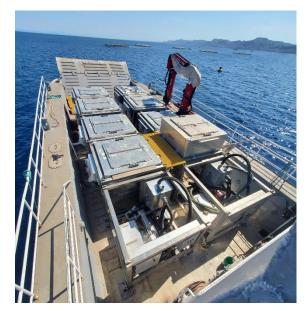
FlowFeeder is an end-to-end feeding solution that can deliver feed to multiple pens from a single, centralized point. It mixes feed pellets with water on the feed vessel and then gently carries the mixture into the pens.
