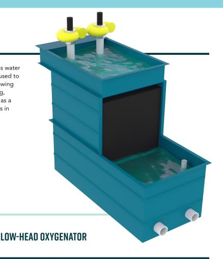
Innovasea's Low Head Oxygenator is a patented, gravity-based solution that injects oxygen into the water while displacing carbon dioxide and nitrogen, achieving more than 100 percent oxygen saturation without the use of electricity. The LHO provides the precise level of oxygen desired while maximizing absorption efficiency. There are two types of LHOs: a round LHO for RAS and partial RAS applications, and a square LHO for raceway and flow-through systems.
